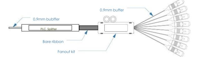
2. Mini-Module PLC Splitter (Only for 0.9mm fiber direct output without fanout kit)
